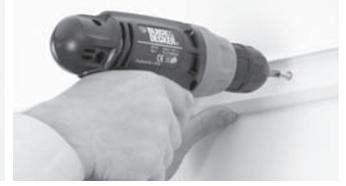
**For the wood screws,** discard the light blue anchor and use a #2 Phillips head screwdriver bit and power drill to tighten the screw. Pulling the wood screw over a bar of soap before using it will make inserting the screw into the wood easier.
