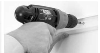
**For the wood screws,** discard the light blue anchor and use a #2 Phillips head screwdriver bit and power drill to tighten the screw. Pulling the wood screw over a bar of soap before using it will make inserting the screw into the wood easier.
